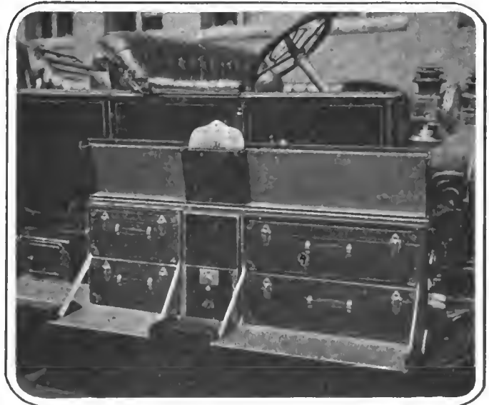
Fig. 10—Method of carrying baggage in waterproof-covered suit cases on the running boards
